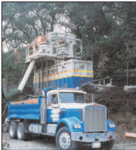
An Akkerman slurry separation plant is perched in the confined area under a large Heritage Oak.
